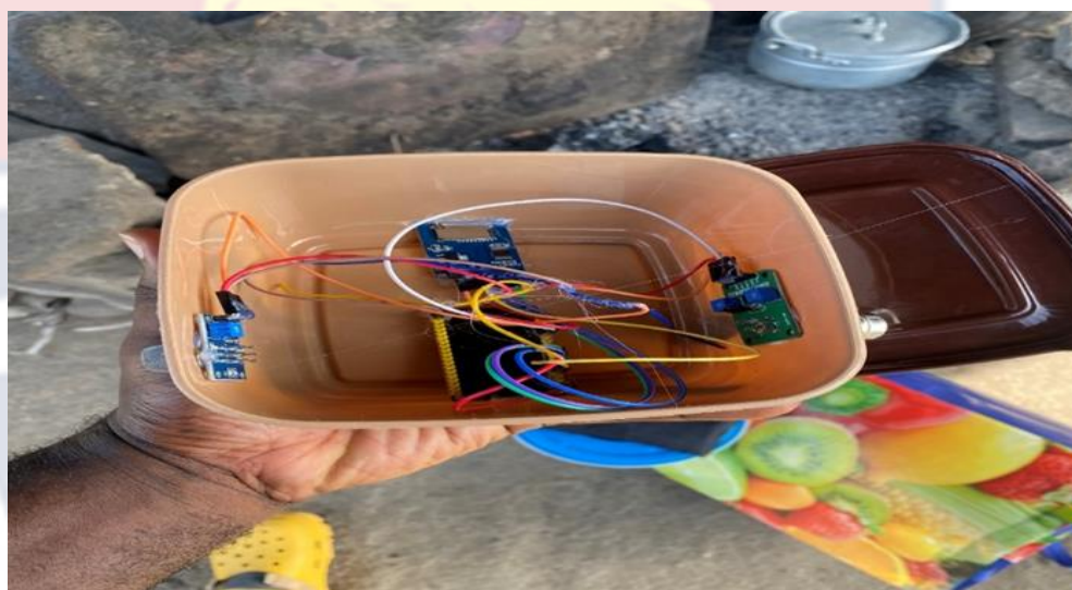
Figure 11: Assembled low-cost air quality sensor.
