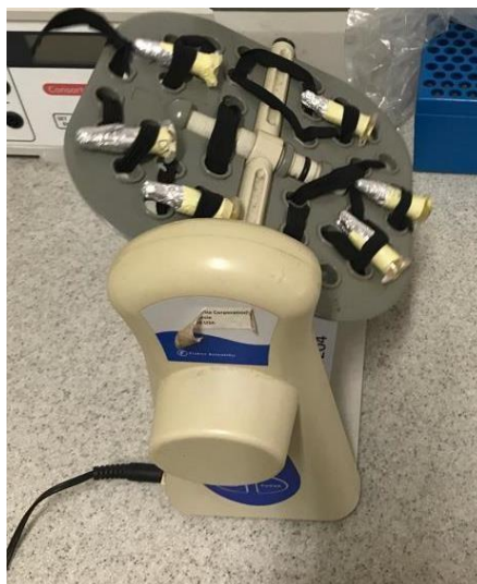
Figure 3.2: Agitation of 100 mg each of 60, 80 and 105 °C synthesized LTA zeolites in 1mg/ml and 2 mg/ml doxorubicin aliquots drug solution to ensure adsorption of drug onto the zeolites.
