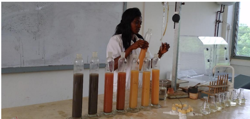
Figure 6: Soil particle size determination using the pipette sampling technique.
