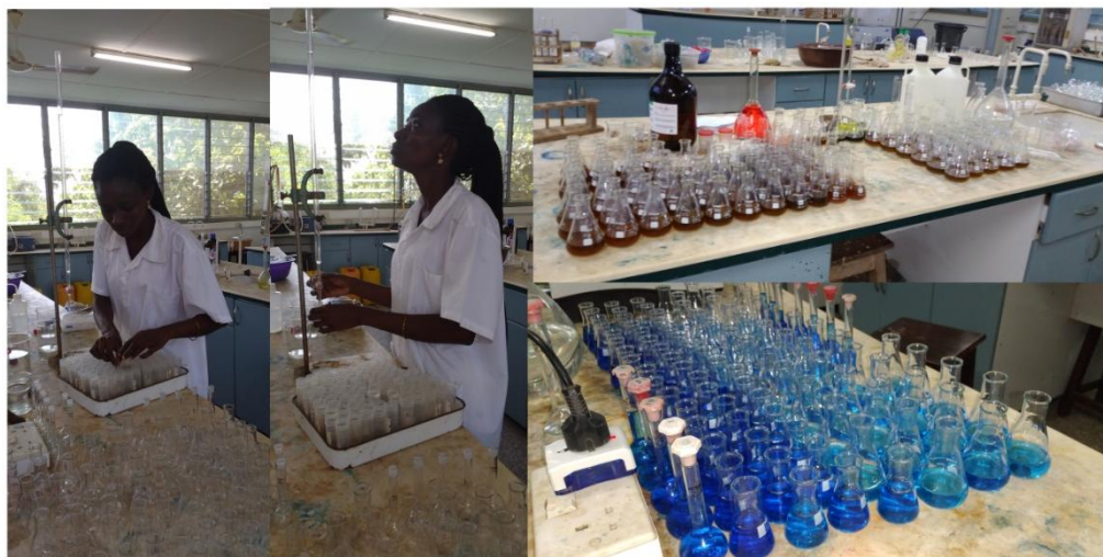
Figure 11: Ammonium and nitrate-nitrogen determination after soil-biochar incubation.
