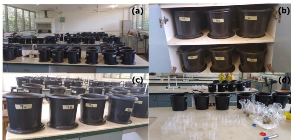
Figure 7: Activities under the incubation experiment; (a) Filled pots (b) incubation of pots and (c, d) soil sampling for analyses during the incubation experiment.
