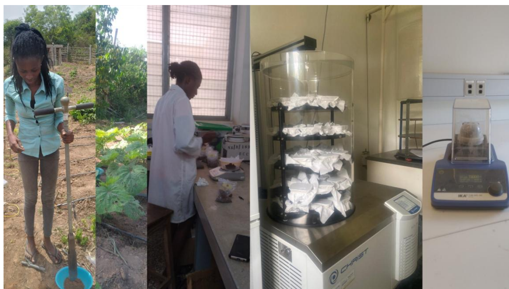
Figure 18: Soil sampling, weighing, freeze-drying and milling for microbial analyses.
