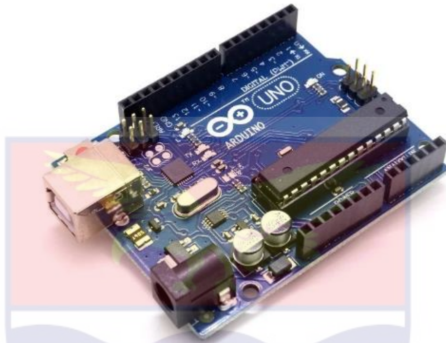
Figure 26: Arduino UNO R3 development board
