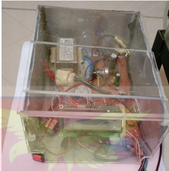
Figure 69: Housing for organ bath power supply circuit board
