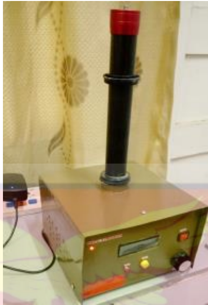
Figure 47: Kymograph electrical base system with a carbon shaft
